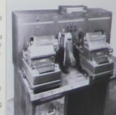
The RED machine, a Type A machine, was used by the Japanese to encrypt diplomatic messages. It was broken by the Army's Signals Intelligence Service in 1936.
